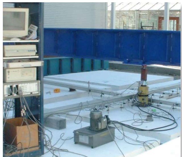
Ground slab testing rig
